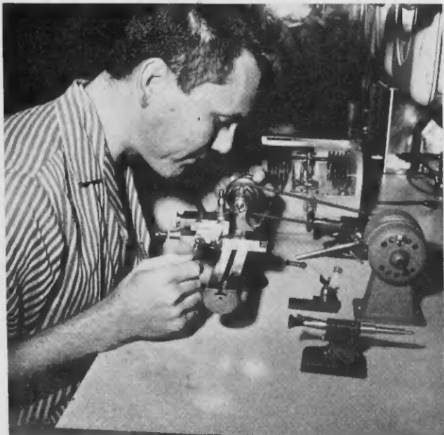
SMALL ELECTRIC motor powers this tiny jeweler's lathe, left, and a sewing machine, right, but a unique air-driven motor, center, is more controllable for laboratory use. An air-driven motor offers precise speed control in critical applications.
